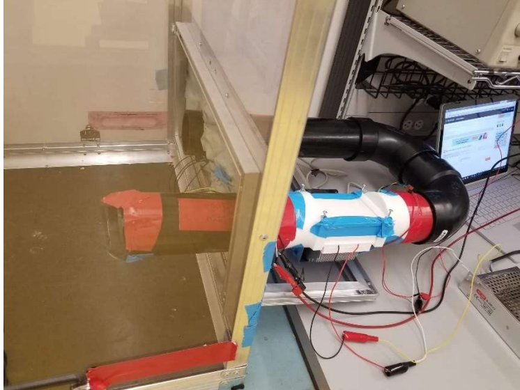
Figure 14: Experimental setup of dehumidifying system in testing chamber
